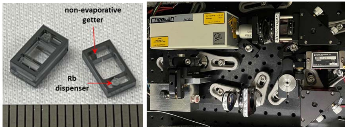
Fig. 1: Chip-scale vapor cell and Rb two-photon spectroscopy setup.
